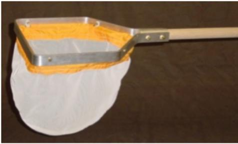
Two common methodologies for sampling macroinvertebrates are kick-netting (sometimes called hand-netting) and Surber sampling (see examples of sampling equipment for each of these techniques below). Which method to use depends on the reason for collecting the samples.
