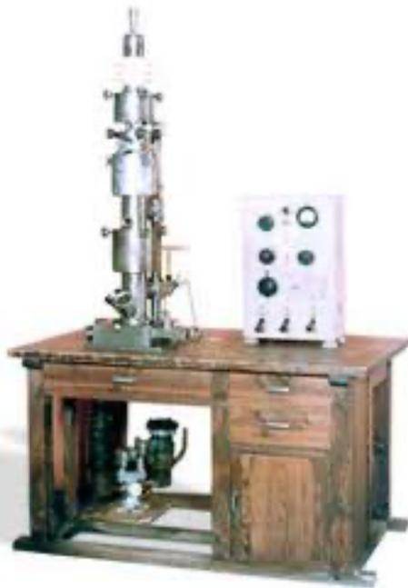
Knoll and Ruska built a transmission electron microscope (TEM) - one that transmits a beam of electrons (as opposed to light) through the specimen. The subsequent interaction of the beam of electrons with the specimen is recorded and transformed into an image. Then, in 1942, Ruska improved on the TEM by building built the first scanning electron microscope (SEM) that transmits a beam of electrons across the specimen.
